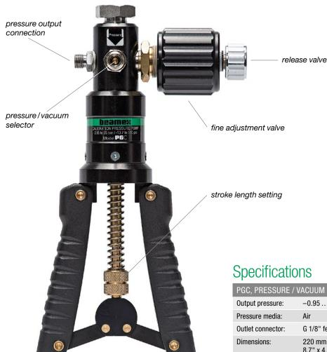
**The PGC** is a hand-operated calibration pump that can be used to generate pressure and vacuum. Using the pressure/vacuum selector you can quickly select if you want to generate pressure or vacuum. The fine adjustment provide means to accurately fine adjust the generated pressure.
