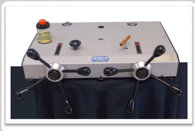
The generator CH2-10000B with kit dead weight tester
